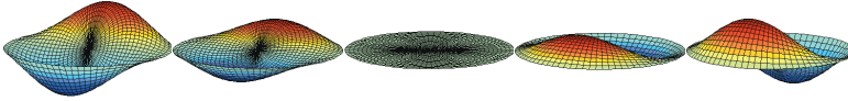
Figure 3.15 Oscillation sequence of the vibrating sheet with a diameter of the sheet as the symmetry axis.
