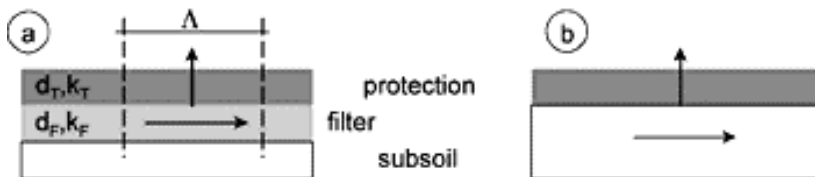
Figure 8-4 Definition leakage length
