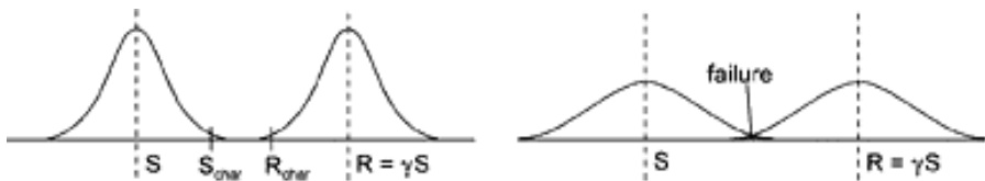
Figure 10-4 Equal overall safety coefficient with different probability distributions
